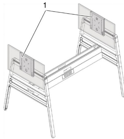
Figure 27 Monitor bracket on low arch attachment, permissible attachment
